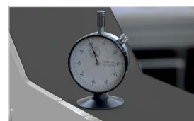
Rollers pressure gauge
