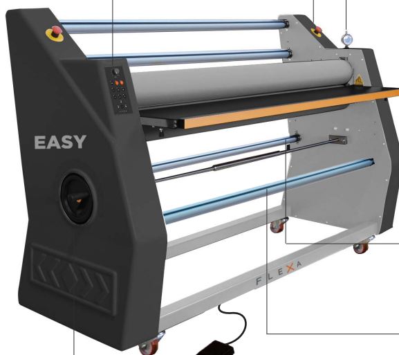
Feeding command by control panel or foot switch (hands free operation)
