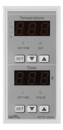
The central controller allows for setting the desired temperature (°C and °F), as well as the press duration in seconds.
