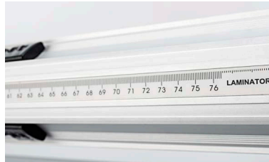
Millimeter scale on each shaft for the right positioning of the media
