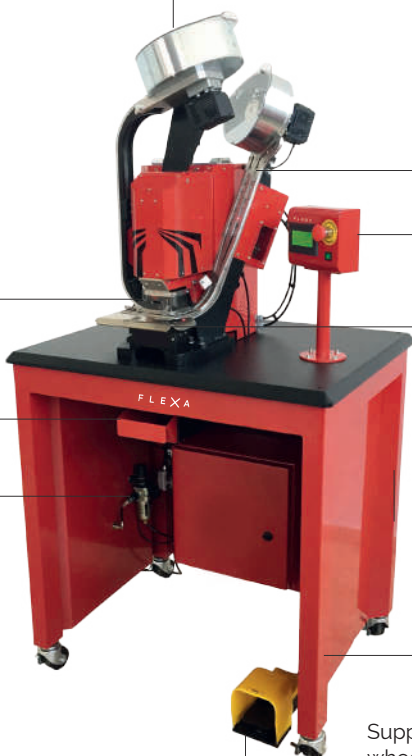
Command with foot pedal (hands free operation)
