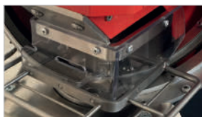
Working area protected by transparent guard
