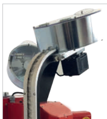
Large hoppers for eyelets and washers
