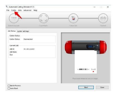
Insert a blank sheet of paper into the vinyl cutter, as requested by DrawCut Pro. Also, the
